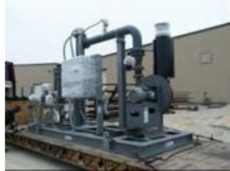
Ammonia Flow Control Package Customer: Sunoco Refinery
